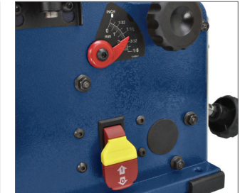
DEPTH SCALE AND SAFETY ON/OFF SWITCH
